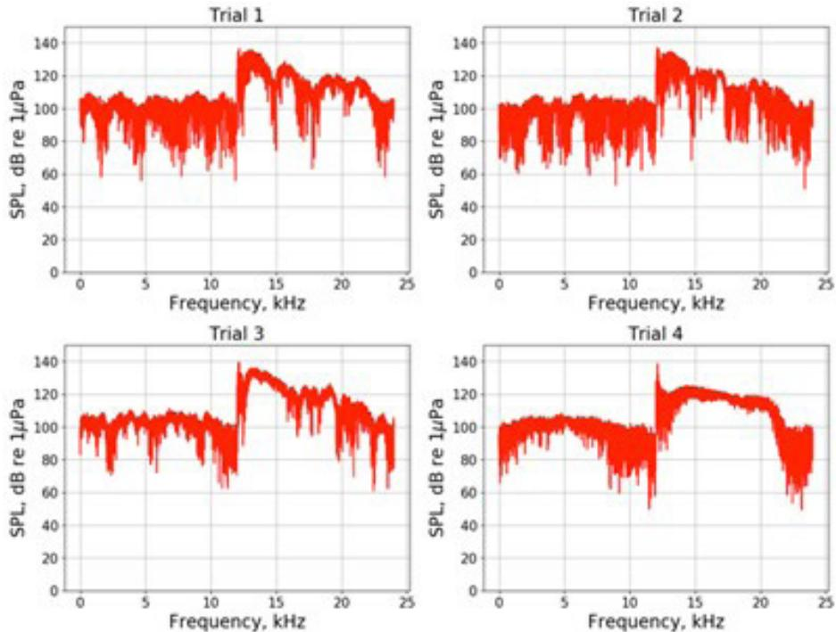
**Figure 3.** Sound pressure level (dB re 1  $\mu$ Pa) from the simulated explosions.
