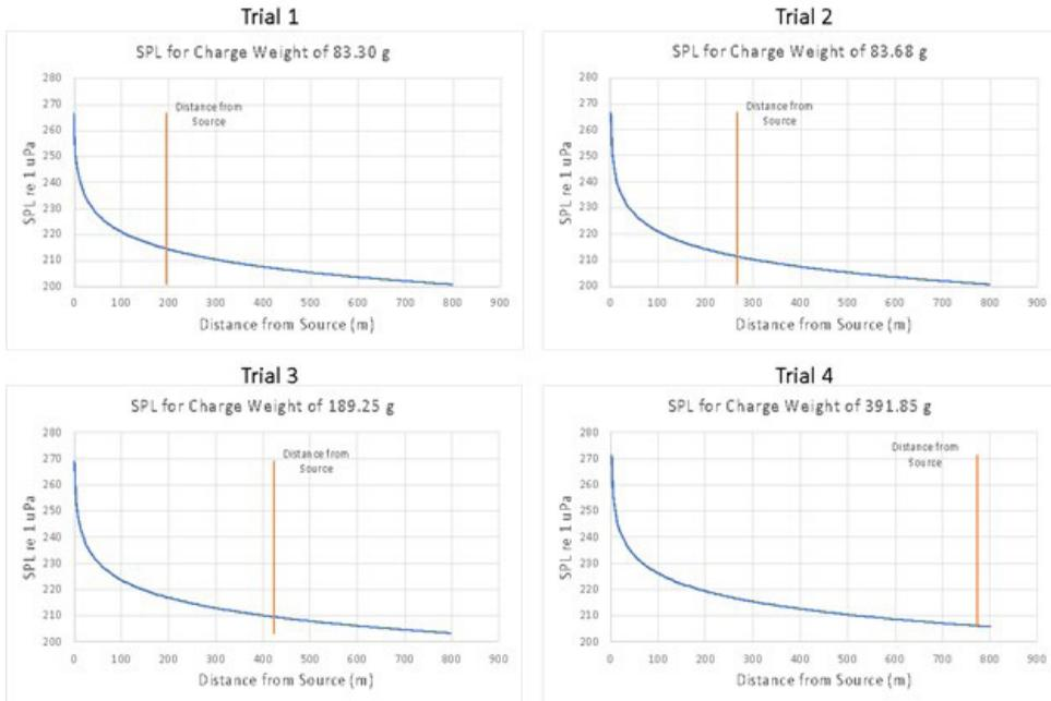
**Figure 4.** Theoretical peak incident pressure based on estimated charge weight.
