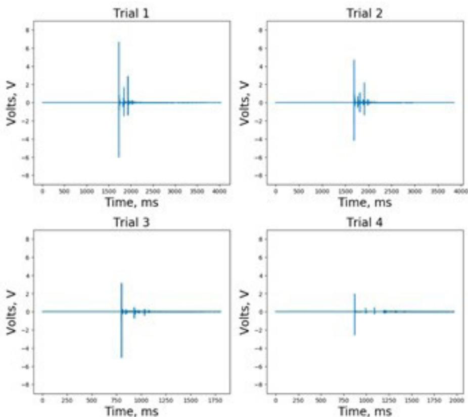
**Figure 1.** Raw signals (in Volts) recorded by the hydrophone during the simulated explosions.
