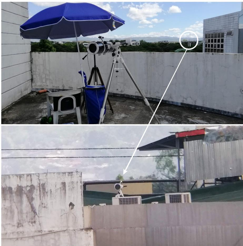
**Figure 5.** The actual DOAS set-up used in the experiment which shows the detector telescope set-up in EEEI (top), and the emitter telescope in NIP as seen through the detector telescope's eyepiece (bottom).
