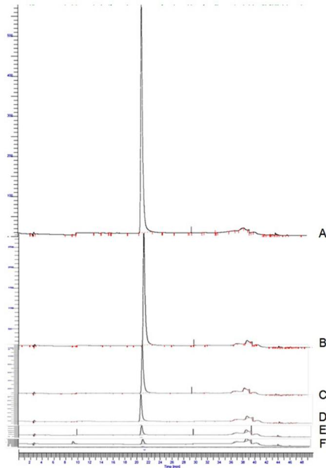
Figure 4. Overlay of chromatograms of the quercetin standard solutions analyzed using the optimized HPLC method: (A) 124.00 µg/mL; (B) 62.00 µg/mL; (C) 31.00 µg/mL; (D) 15.50 µg/mL; (E) 7.44 µg/mL; and (F) 3.72 µg/mL
