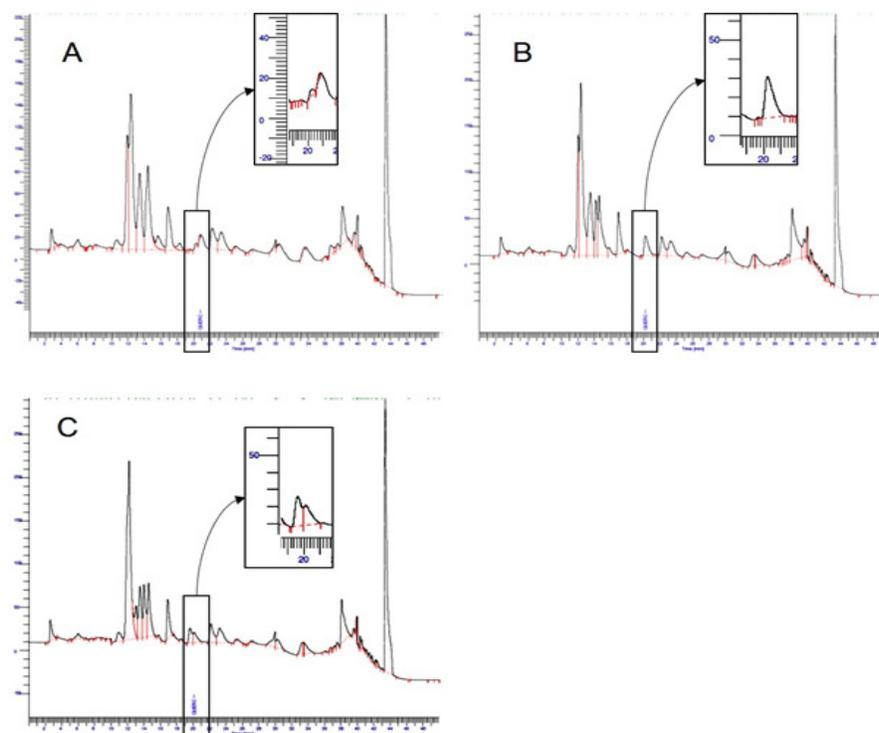
Figure 3. Chromatograms of sambong solutions run in different mobile phase compositions. The mobile phase composition was changing to 100% methanol in a 50-minute gradient program starting with the following solvent combinations: (A) 25:75 methanol:0.5%  $\text{H}_3\text{PO}_4$ ; (B) 25:75 methanol:0.5%  $\text{H}_3\text{PO}_4$  with 0.2% triethylamine; and (C) 25:75 methanol:0.5%  $\text{H}_3\text{PO}_4$  with 0.5% triethylamine.
