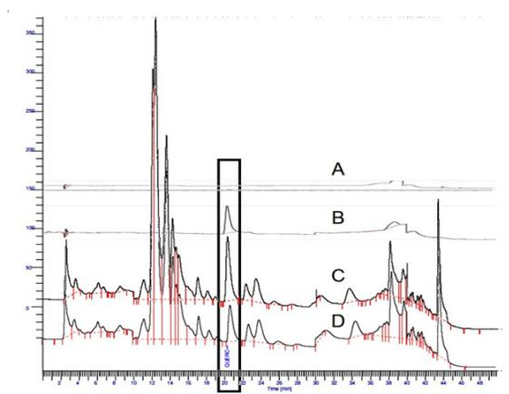
Figure 2. Overlay of chromatograms of solutions that were treated in the SPE tube in the same manner: (A) methanol; (B) quercetin standard solution (15.62  $\mu\text{g/mL}$ ); (C) sambong solution spiked with 15.62  $\mu\text{g/mL}$  quercetin standard; and (D) unspiked sambong solution
