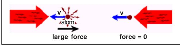
Fig. 1. The formation of optical molasses in one dimension using two laser beams. To account for the Doppler shift of resonance frequency, red-detuned laser beams are used.
