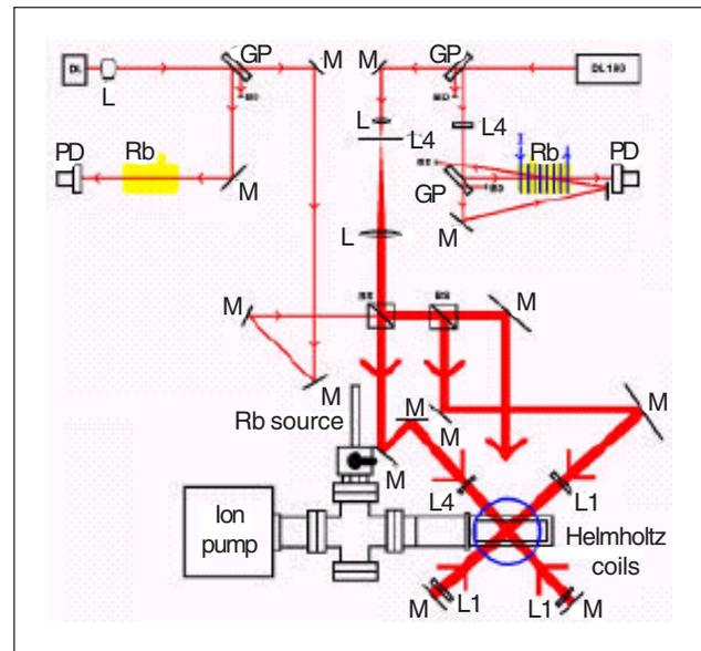
Fig. 2. Experimental setup for laser cooling and trapping of Rb atoms. The upper right part shows the saturation spectroscopy setup for the trapping laser. A current running through a coil wrapped around the Rb vapor cell produces a magnetic field to induce a Zeeman shift of the cooling transition. The upper left part shows the saturation spectroscopy setup for the repumper laser. The lower part shows the trapping cell with the anti-Helmholtz coils.
