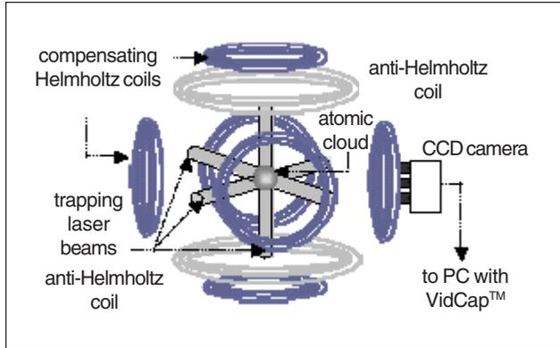
Fig. 3. Experimental setup for the measurement of temperature for atoms expanding in optical molasses when the current through the anti-Helmholtz coils is switched off.
