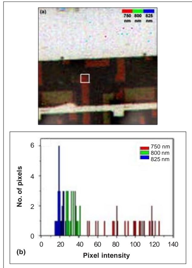
Fig. 3. (a) Composite image (area of 200x200 μm<sup>2</sup>) of the photodiode array generated from the OBIC images taken at 750, 800, and 825 nm. The OBIC images are masked each in red (750 nm), green (800 nm), and blue (825 nm). The composite image reveals the optical response of the semiconductor with varying wavelengths as shown when (b) a histogram of a particular region [bounded area in (a)] is generated.
