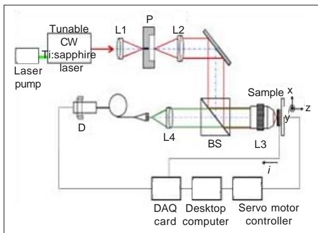
Fig. 1. The optical setup. The tunable Ti:Sapphire laser is pumped by a solid-state laser. The laser output is spatially filtered, collimated, and focused on the sample by an objective system. The reflected signal is detected by a PMT. OBIC measurements are directly obtained by the data-acquisition card.
