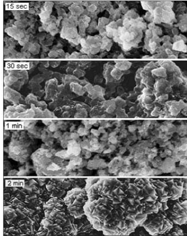
Fig. 5. SEM images of  $\text{MgB}_2$  films at 8000x.
