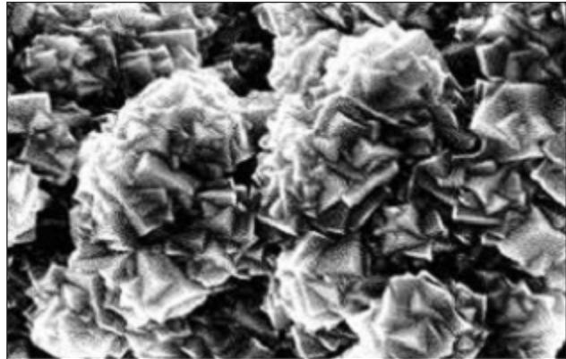
Fig. 6. Enlarged SEM image of  $\text{MgB}_2$  film deposited for 2 min.
