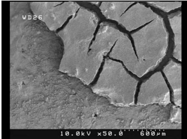
Fig. 1.  $\text{MgB}_2$  film deposited on silver substrate.
