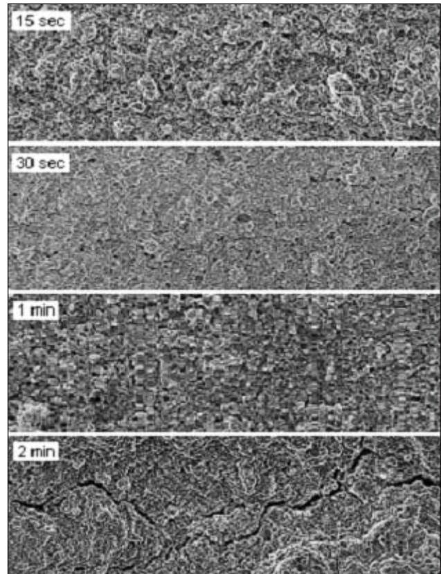
Fig. 2. Deposition surface of  $\text{MgB}_2$  films (400x).
