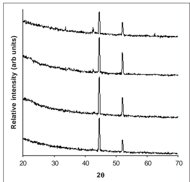
Fig. 3. XRD patterns of  $\text{MgB}_2$  deposited on Mo by EPD.
