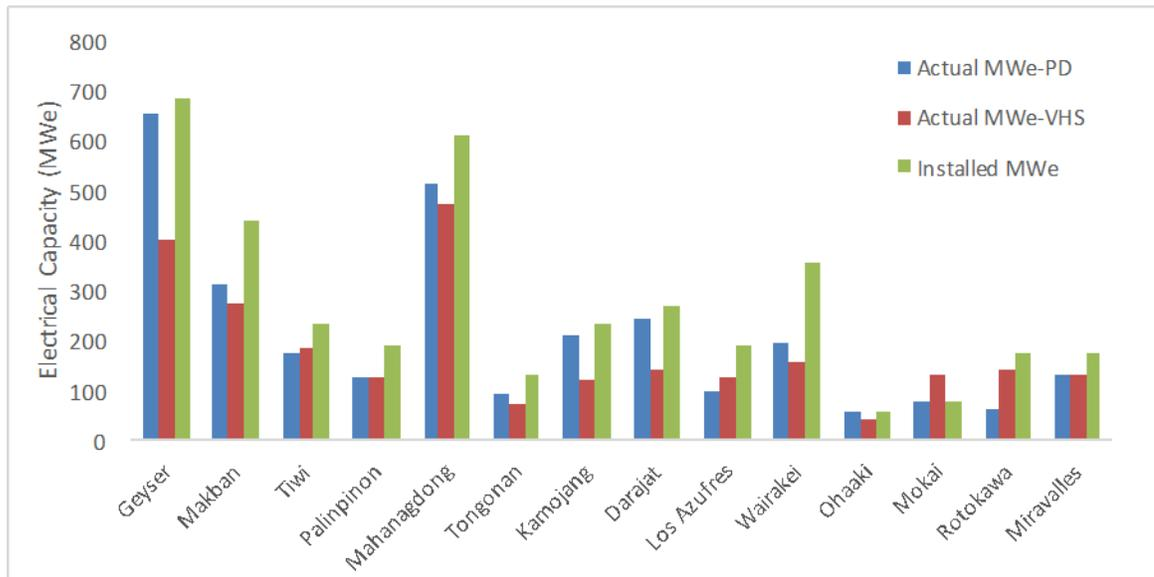
**Figure IV-1** Calculated electrical capacity in MWe based on power density and volumetric stored heat calculations
