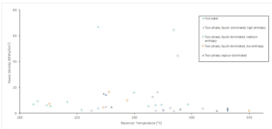
**Figure III-3** Power density plot in terms of the nature of the geothermal system
