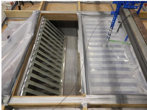
**Figure 9.** Pull-through failure of a sample
