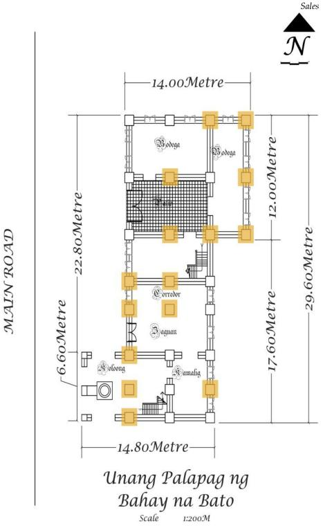
**Figure 16:** Possible ground floor plan of Structure A. Coloured columns are the columns found still standing in the site (Illustration by Angelus Sales).
