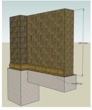
**Figure 19:** A 3d modelling of how the exterior wall may have been constructed (Illustration by Angelus Sales).
