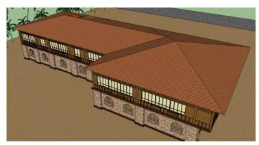
**Figure 27:** A 3d modelling of Structure A showing the hipped roof (Illustration by Mary Nolyn Ventura).
