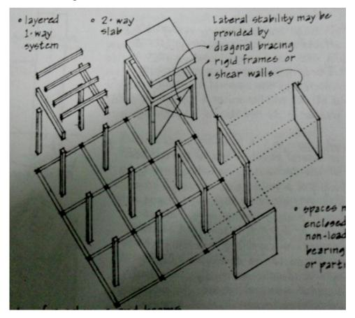
**Figure 15:** An illustration of a linear structural system (Source: Building Construction Illustrated, 2<sup>nd</sup> edition. This material is reproduced with permission of John Wiley & Sons, Inc.).
