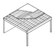
**Figure 24:** An illustration of a floor framing system consisting of floor joists and floor boards (Source: Building Construction Illustrated, 4<sup>th</sup> edition. This material is reproduced with permission of John Wiley and Sons, Inc.).
