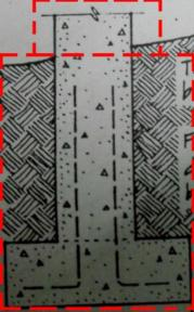
**Figure 11:** An illustration of a modern spread footing foundation. (Source: Building Construction Illustrated, 2<sup>nd</sup> edition. This material is reproduced with permission of John Wiley and Sons, Inc.). The red dash lines are outline of the spread footing used for Structure A.
