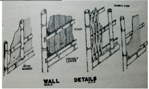
**Figure 4:** Examples of different types of materials used for walls in a bamboo nipa hut (Source: Balai Vernacular: Images of Filipino Private Space. Published with the permission from Cultural Center of the Philippines).
